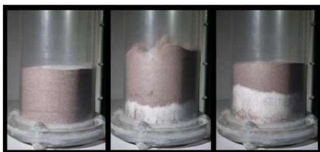
Fig. 2. Snapshots of fluidized bed in before, during and after the segregation process for bed height of 9 cm, flotsam-rich composition and inlet air velocity of 0.10 m/s
