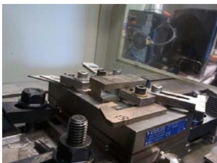
Fig. 1. Work piece clamped onto dynamometer
