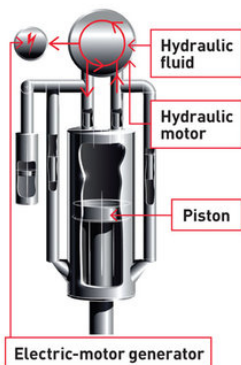
Fig.5 Hydraulic transmission regenerative damper
