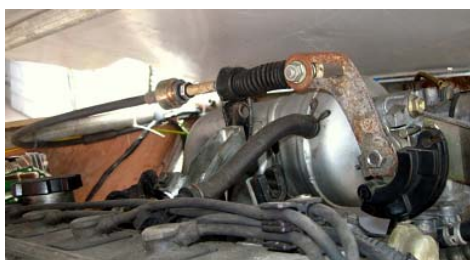
Fig. 25 Mechanical linkage of the carburetor
