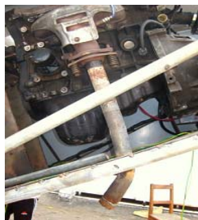
Fig. 26 Exhaust pipe modification
