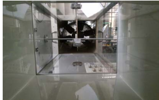
Fig. 13 Scale model in wind tunnel
