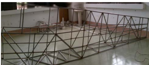
Fig. 18 Fuselage skeleton structure fabrication
