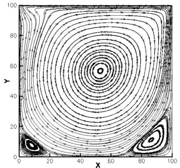
Fig. 2. Streamlines of lid-driven cavity at Re=1000
