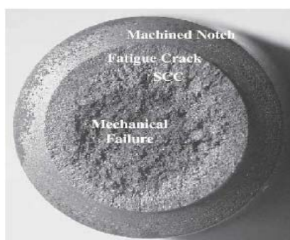
Figure 5 Overall fracture surface of a AISI 4140 Steel CNT specimen tested in 80^\circ\text{C} NaOH solution.
