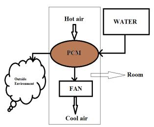
Fig 2 Overview of the cooling system
