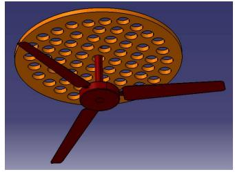
Fig 1 Design of PCM with Ceiling fan
