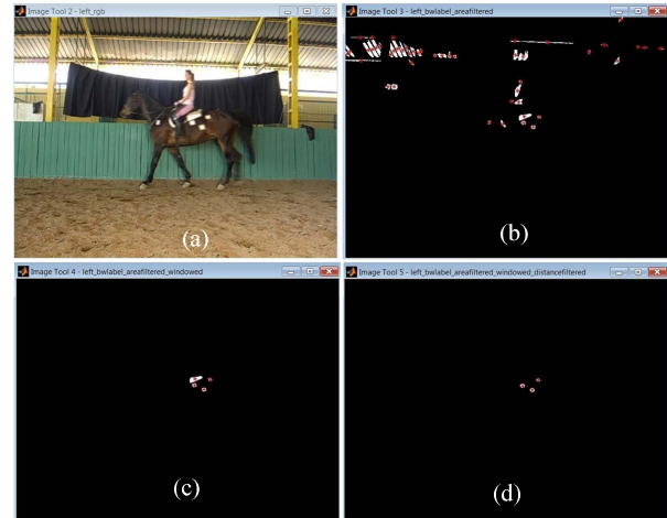
Fig. 4. The stages of filtering methods applied to Horse 3 - walk. The centers of the regions are shown by red asterisk (a) The original RGB color image (b) The area filtered black and white image (c) The regions in the dynamic window (d) The distance and cross product filtered image
