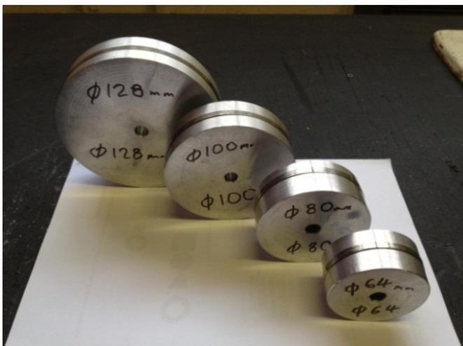
Fig.4 Test samples checking for roundness & size
