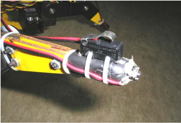
Fig. 2. Push button attached to the leg.
