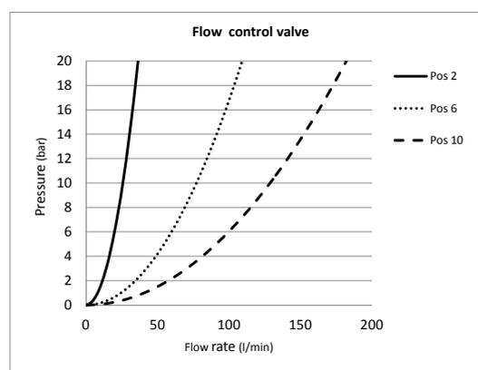
Fig. 7. Flow control valve characteristics.
