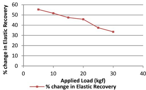
Figure 3: Plot of applied load against springback and curvature
