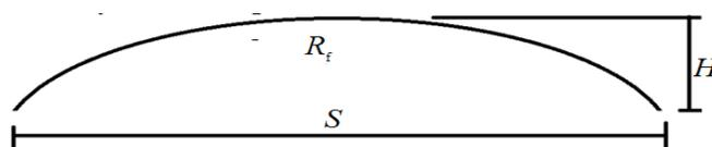
Figure 4: Schematic showing the parameters for calculating the radius of curvature
