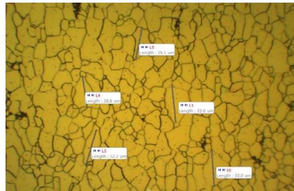
Figure 6: Typical micrograph of the measured grain sizes (10kgf load)
