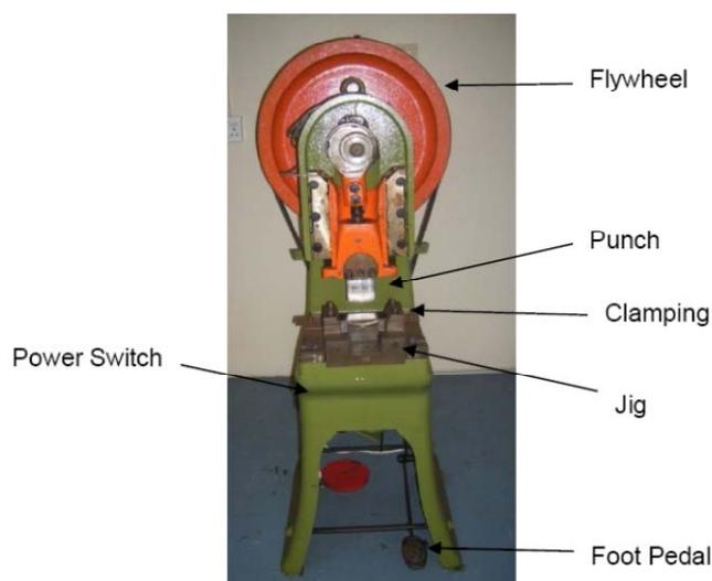
Figure 3: Experimental set-up for mechanical bending process
