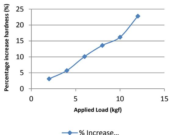
Figure 9: Graph of applied load against hardness
