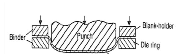
Figure 1: Schematic of Mechanical forming process [4]
