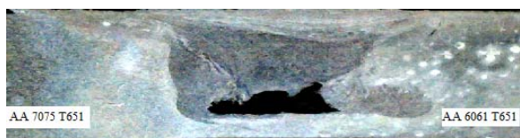
Fig.3 (c): Macrograph of weld produced at 900 rpm and 100 mm/min for simple square profile.
