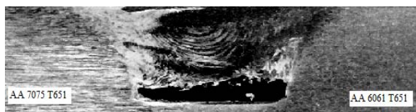
Fig.3 (a): Macrograph of weld produced at 900 rpm and 90 mm/min for taper cylindrical threaded profile
