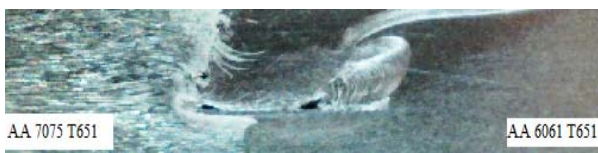
Fig.3 (d): Macrograph of weld at 20X produced at 900 rpm and 110 mm/min for Taper Square threaded profile.
