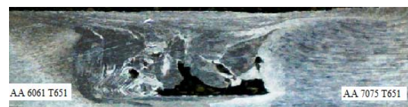
Fig.4 (d): Macrograph of weld produced at 1000 rpm and 110 mm/min for simple square profile.
