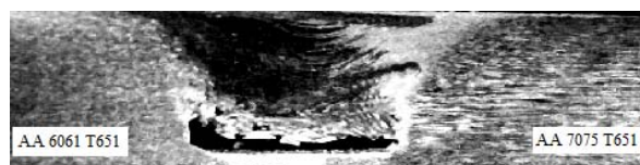
Fig.4 (b): Macrograph of weld produced at 1000 rpm and 100 mm/min for taper cylindrical threaded profile.
