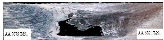
Fig.2 (c): Macrograph of weld produced at 800 rpm and 110 mm/min for simple square profile
