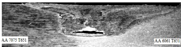
Fig.3 (b): Macrograph of weld produced at 900 rpm and 90 mm/min for Taper Square threaded profile
