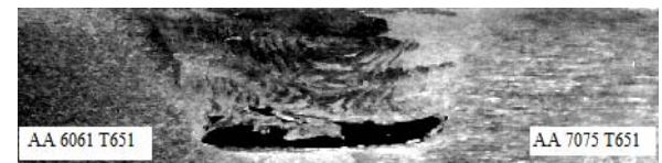
Fig.2 (b): Macrograph of weld produced at 800 rpm and 100 mm/min for taper cylindrical threaded profile
