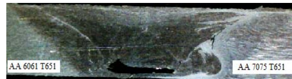
Fig.2 (a): Macrograph of weld produced at 800 rpm and 90 mm/min for simple square profile
