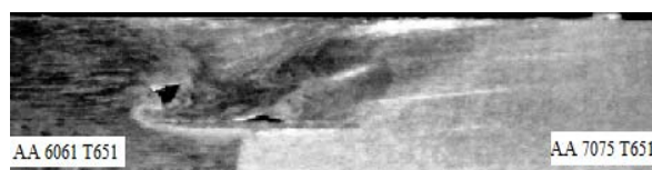
Fig.4 (c): Macrograph of weld produced at 1000 rpm and 100 mm/min for Taper Square threaded profile.
