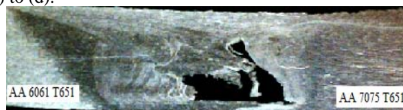
Fig.4 (a): Macrograph of weld produced at 1000 rpm and 90 mm/min for simple square profile.
