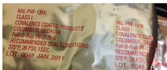
Fig. 3. Material bag used for printing.
