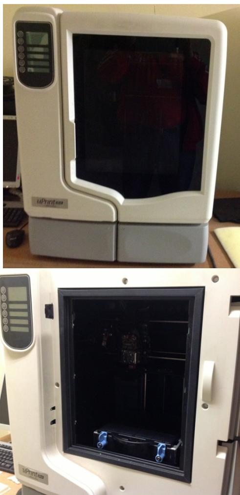
Fig. 2. Rapid prototype machine, exterior and interior.
