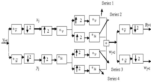
Fig. 1. Block diagram of Oversampling Technique using DWT
