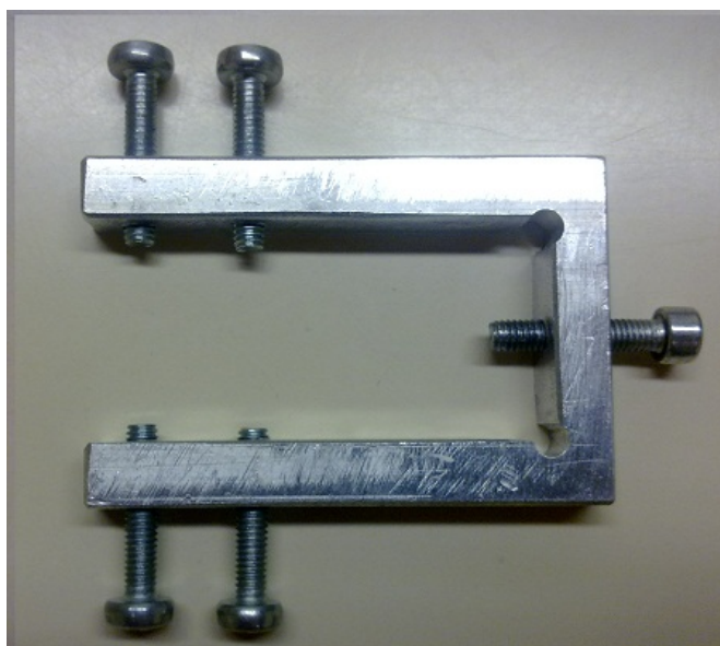
Figure 4. Device used to hold the ultrasonic transducers and maintain a constant pressure during the test.
