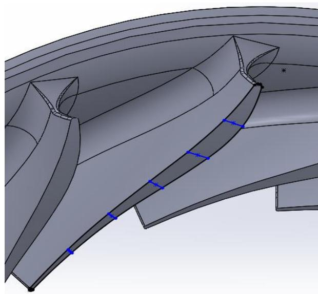
Fig. 8. Determination of blade thickness
