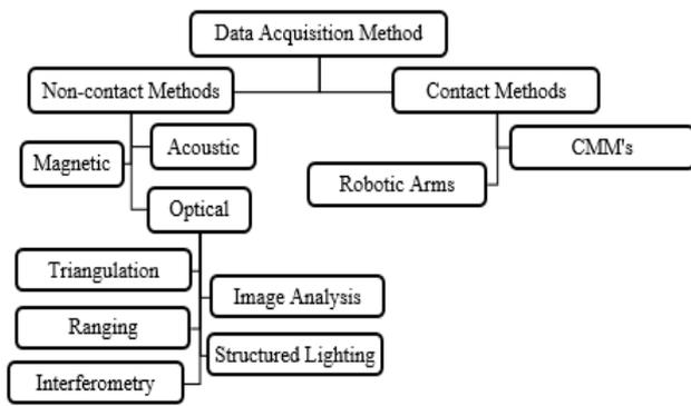
Fig. 2. Classification of data acquisition methods
