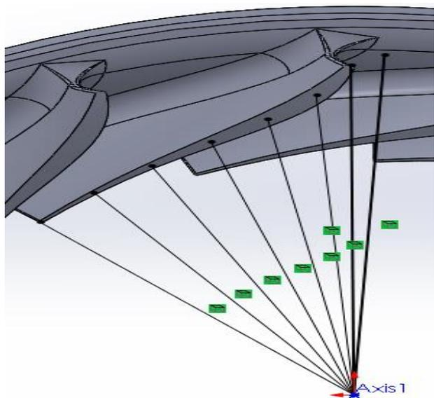
Fig. 7. Determination of theta angle
