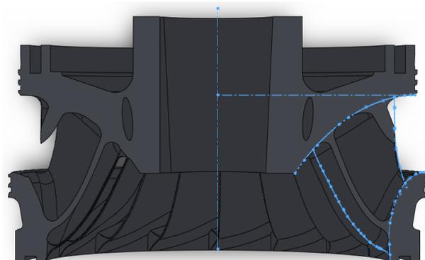
Fig. 5. Determination of meridional contour
