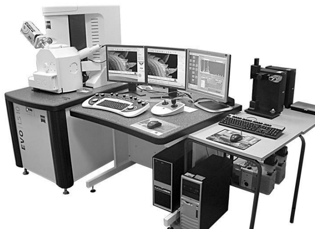
Fig. 2. Pictorial diagram of the SEM-EDXA
