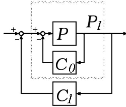
Fig. 4. Two-Stage Compensator Design ( $y_2$  to  $u_2$ ).
