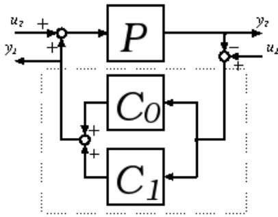
Fig. 5. Composite Stabilized Feedback with  $c_0$  and  $c_1$ .
