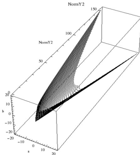
Fig. 13. Norms of output signal  $y_2$  based on Theorem 3.  $R_1$  form is  $a+bd$ .  $a$  and  $b$  range are  $-20 \leq a, b \leq 20$ .
