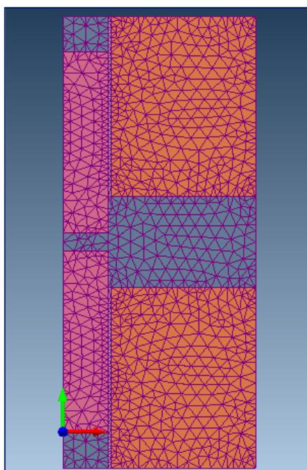
Fig. 2(c) 2-D triangular meshing of the electromagnet
