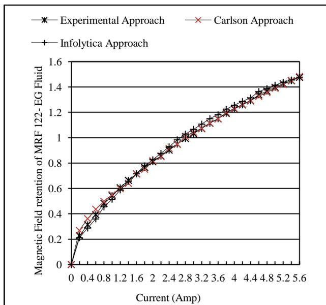
Fig. 5 Comparison of Magnetic Flux Density from Various Approaches
