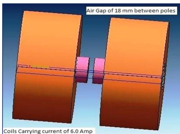
Fig. 2(b) MAG-NET model for simulating Magnetic field
