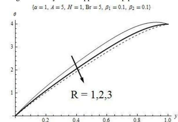
Fig 3: Temperature versus thermal radiation parameter
