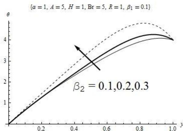
Fig 5: Temperature versus upper wall slip parameter
