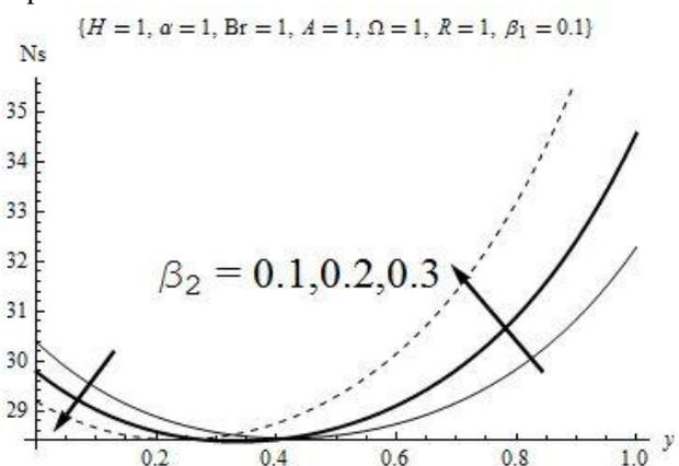
Fig 7: Entropy generation versus upper wall slip parameter
