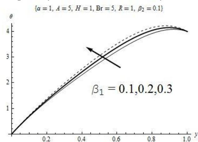
Fig 4: Temperature versus lower wall slip parameter
