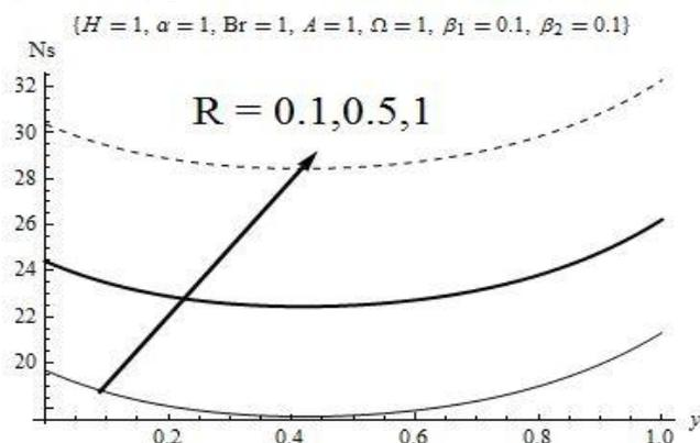
Fig 8: Entropy generation versus Thermal radiation parameter
