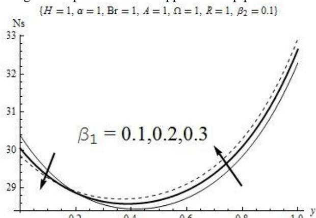
Fig 6: Entropy generation versus lower wall slip parameter
