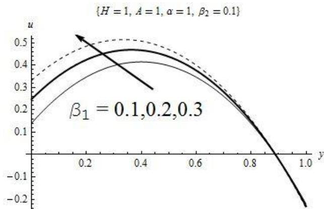
Fig 1: Velocity versus lower wall slip parameter
