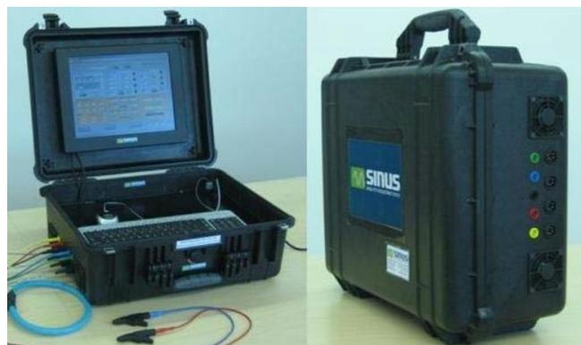
Fig. 1. Power quality analyser developed by GEPE - University of Minho.
