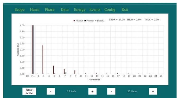
Fig. 11. Harmonics menu: Amplitudes of the harmonics and THD values of the three phases currents.
