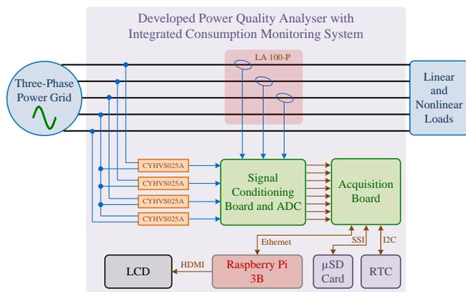
Fig. 2. Block diagram of the developed electrical energy consumption and power quality analysis monitoring system.
