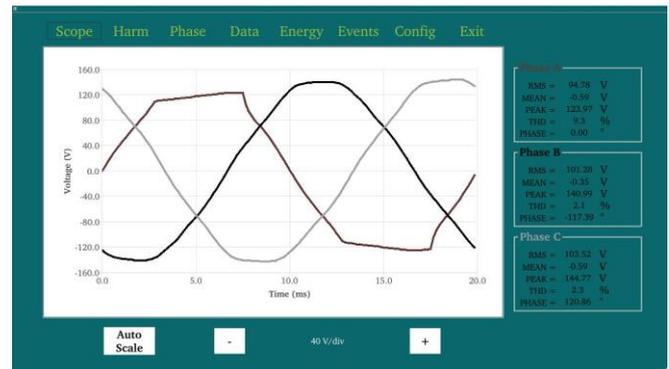
Fig. 9. Scope menu: Waveforms of the three-phase voltages using a nonlinear load.
