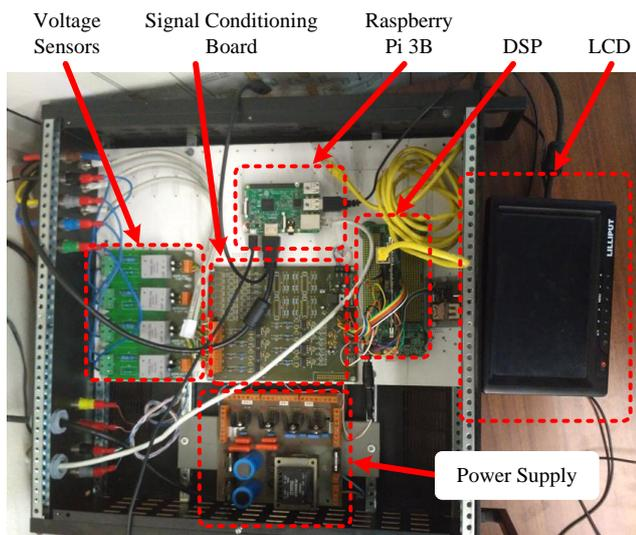
Fig. 4. Developed power quality analyser with integrated electrical energy consumption monitoring system.
