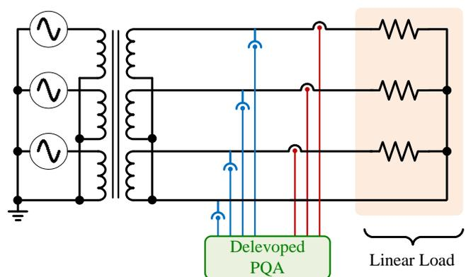
Fig. 6. Electrical diagram of the setup used with a linear load.
