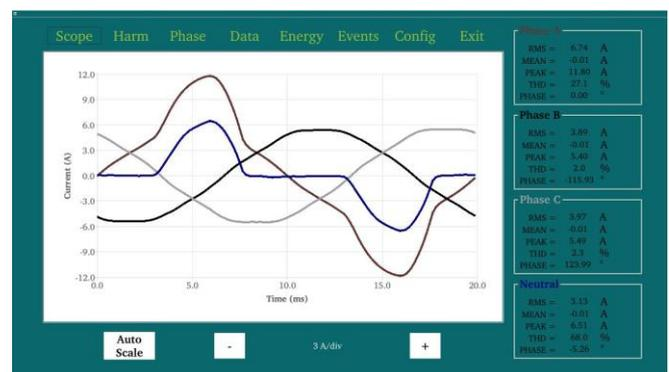
Fig. 10. Scope menu: Waveforms of the three phases currents and neutral current using a nonlinear load.
