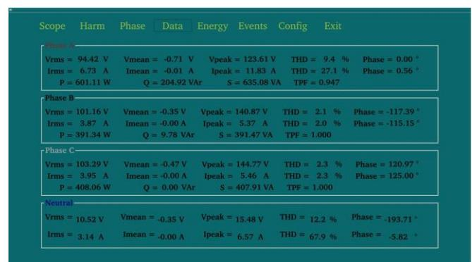
Fig. 12. Data menu: Values of all the measured parameters for the voltages and currents.
