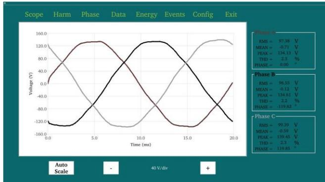
Fig. 7. Scope menu: Waveforms of the three-phase voltages using a linear load.
