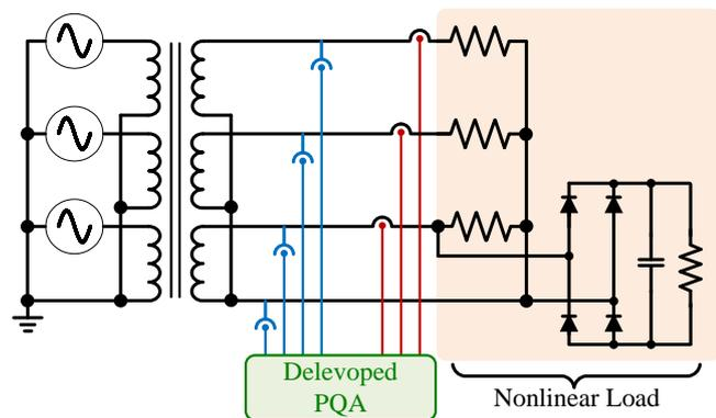
Fig. 8. Electrical diagram of the setup used with a nonlinear load.
