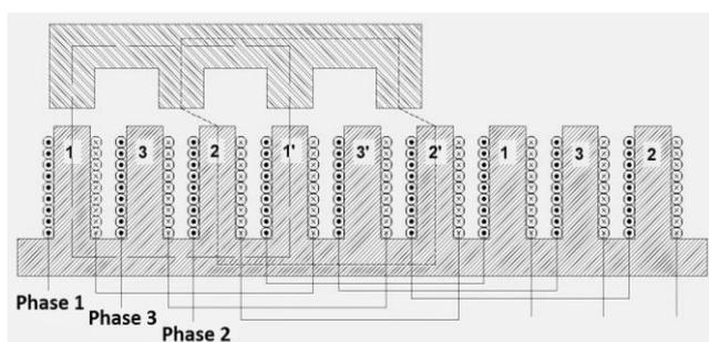
Fig. 1. Cross sectional view of Linear Switched Reluctance Motor
