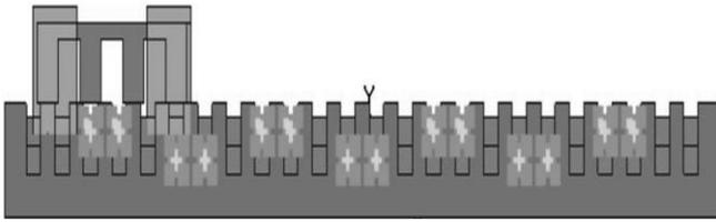
**Fig. 4.** Linear switched reluctance motor design for MagNet simulation
