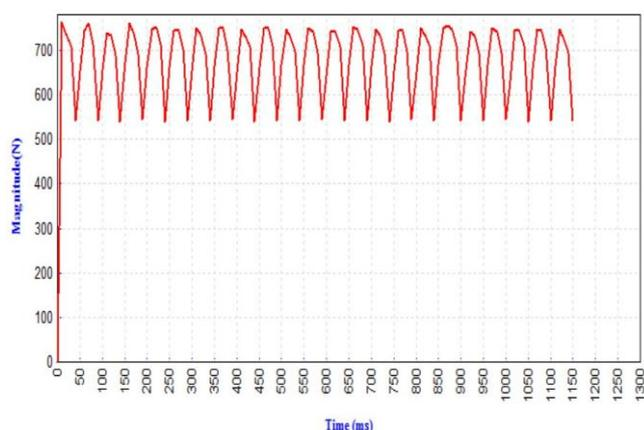
**Fig. 12.** Force generated on translator made up of soft pure Iron with semi-enclosed slots
