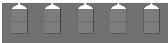
Fig. 10(a). Stator design with semi-enclosed slots using MagNet Software
