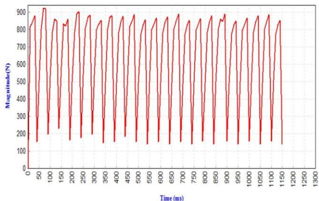
Fig. 8. Force generated on translator made up of soft pure Iron with open slots
