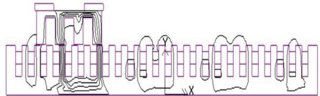
**Fig. 6(b).** Open slot design of stator with flux function plot using MagNet software
