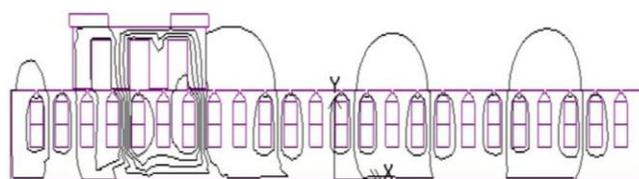
Fig. 10(b): Semi-enclosed slot design of stator with flux function plot using MagNet software
