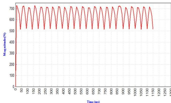
Fig. 11. Force generated on translator made up of Stainless Steel with semi-enclosed slots
