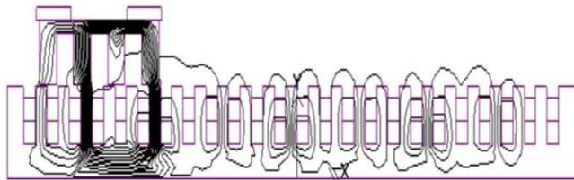
**Fig. 5.** Flux lines when translator is under influence of excited coils
