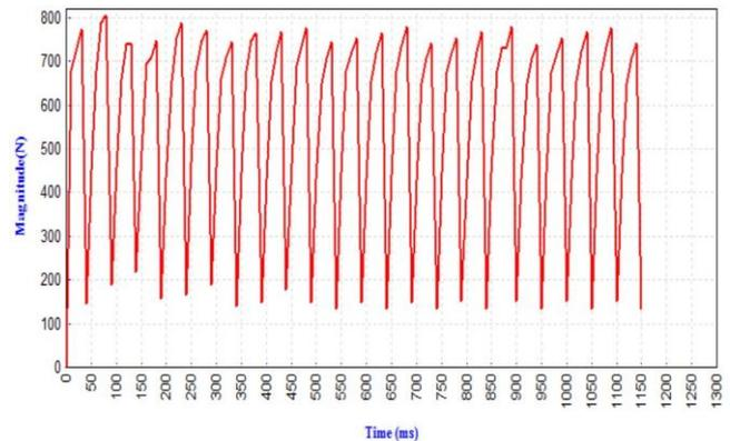
**Fig. 7.** Force generated on translator made up of Stainless Steel with open slots
