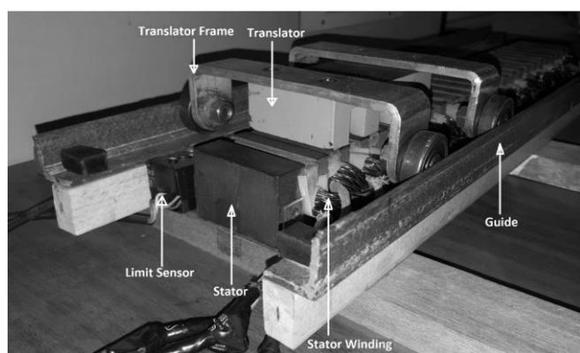
Fig. 9. Prototype of LSRM
