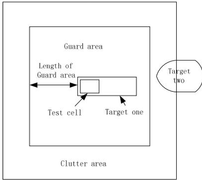
Fig. 1. Reference window for CFAR detection
