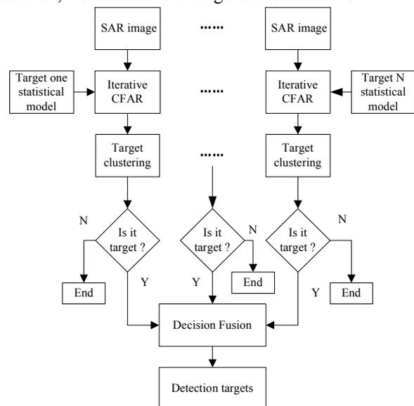
Fig. 3. Flow of multi-target detection
