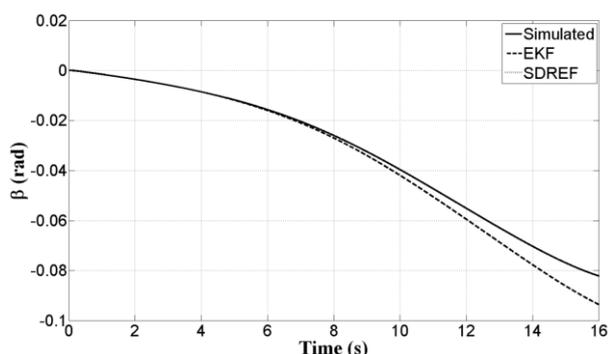
Fig. 2. Sideslip angle – steering pad manoeuvre.
