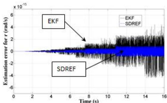
Fig. 7. Estimation error for yaw rate – steering pad manoeuvre.
