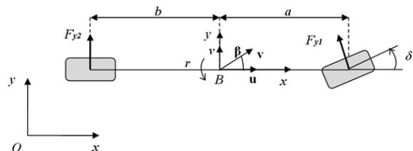
Fig. 1. Reference frames and vehicle model.
