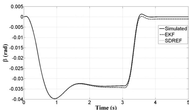
Fig. 8. Sideslip angle – double lane change manoeuvre.
