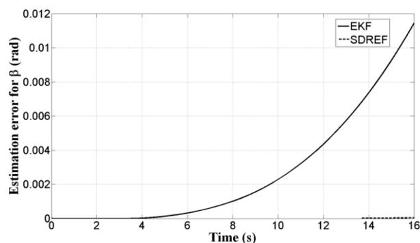
Fig. 3. Estimation error for sideslip angle – steering pad manoeuvre.
