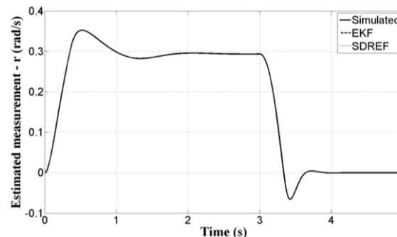
Fig. 12. Yaw rate – double lane change manoeuvre.
