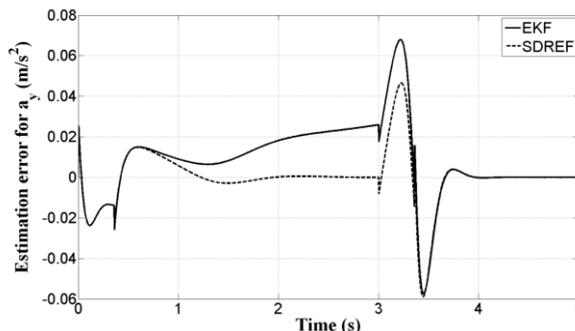
Fig. 11. Estimation error for lateral acceleration – double lane change manoeuvre.
