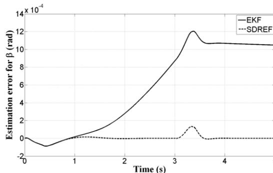
Fig. 9. Estimation error for sideslip angle – double lane change manoeuvre.
