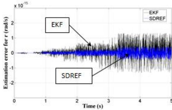
Fig. 13. Estimation error for yaw rate – double lane change manoeuvre.
