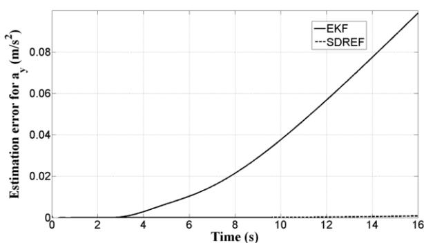
Fig. 5. Estimation error for lateral acceleration – steering pad manoeuvre.
