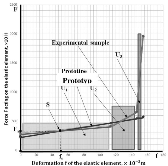
Fig. 1. Comparison of theoretical and experimental results
