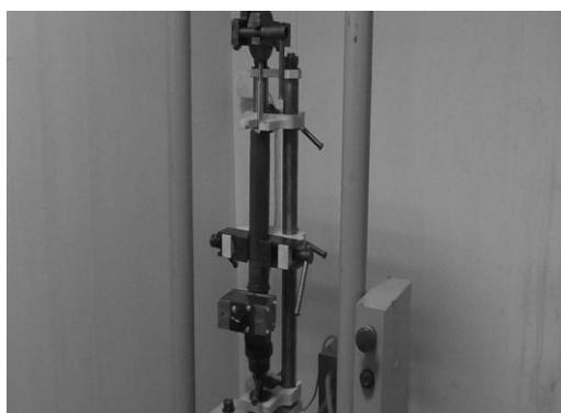
Fig. 10. Experimental stand for the shock absorber test
