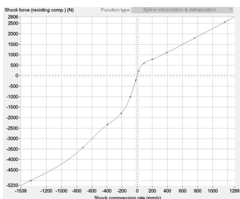
Fig. 11. Experimental characteristic of shock absorber
