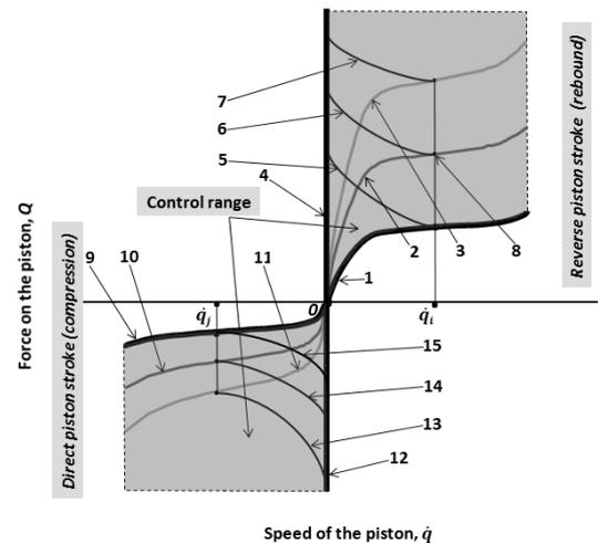
Fig. 5. Operating characteristics of the shock absorber at variable operating influence
