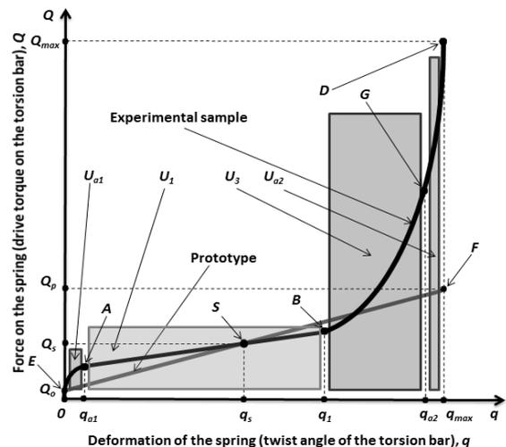
Fig. 8. Operating characteristics of the elastic element based on the availability of the adaptive shock absorber (the second variant)
