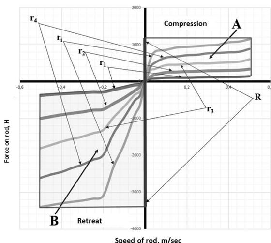
Fig. 2. Work characteristic of adaptive shock absorber
