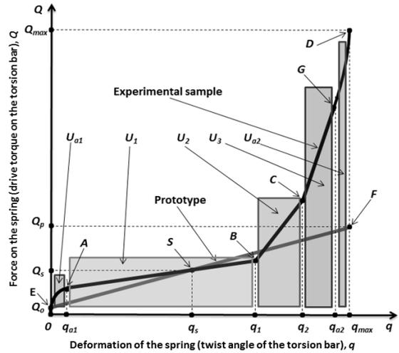
Fig. 7. Operating characteristics of the elastic element based on the availability of the adaptive shock absorber (the first variant)
