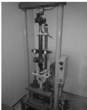
Fig. 9. Experimental stand for the shock absorber test
