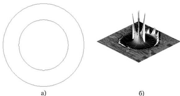
Fig. 1 Picture wave fronts (a) and the amplitude of movements (b) for siltstone under the action of a concentrated force
