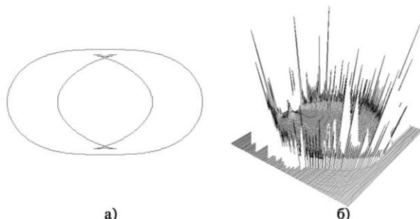
Fig. 3 Picture wave fronts (a) and the amplitude of movements (b) for Zn under the action of a concentrated force
