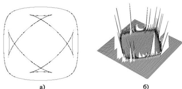
Fig. 4 Picture wave fronts (a) and the amplitude of movements (b) for topaz under the action of a concentrated force
