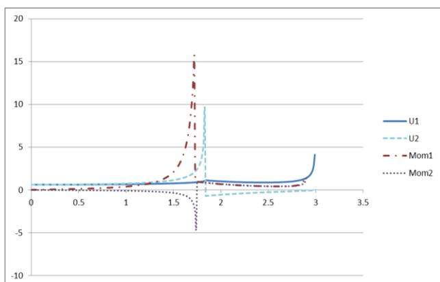
Fig.6 Components of the Green's tensor for siltstone under the action of concentrated forces and moments at  $t = 3$
