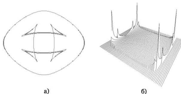
Fig. 5 Picture wave fronts (a) and the amplitude of movements (b) for potassium pentaborate under the action of a concentrated force
