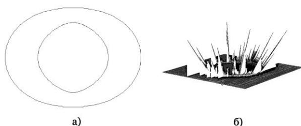
Fig. 2 Picture wave fronts (a) and the amplitude of movements (b) for aragonite under the action of a concentrated force
