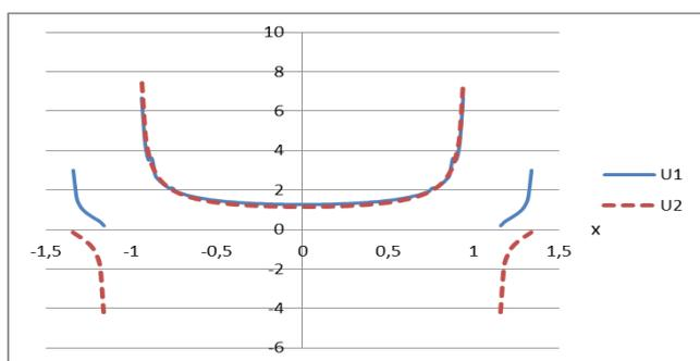
Fig. 2 Components of the Green's tensor for topaz under the action of a concentrated force
