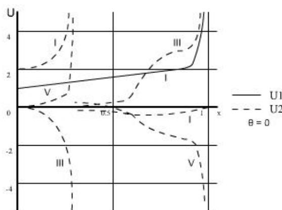
Fig.8 Components of the Green's tensor for potassium pentaborate under the action of concentrated forces
