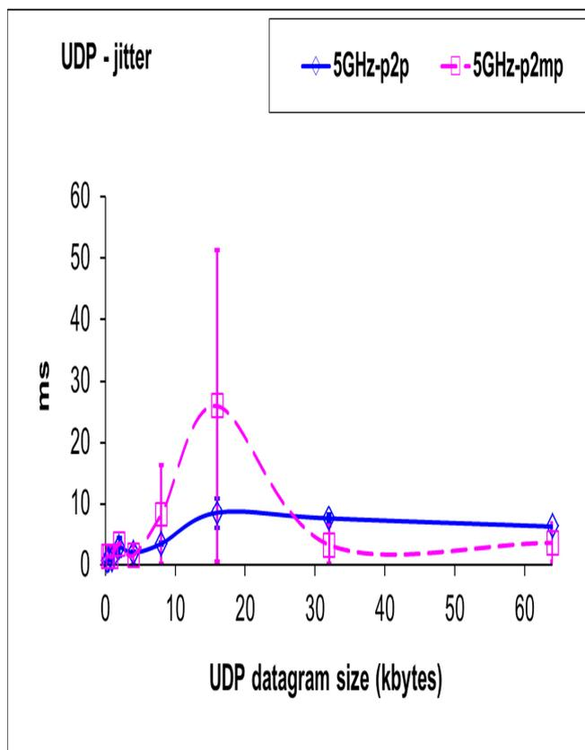
Fig. 4- UDP - jitter versus UDP datagram size. WEP links.
