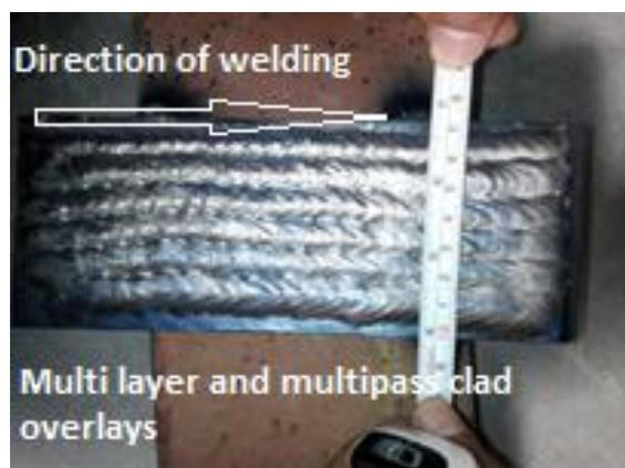
Figure 3 Multi-layer and multi-pass clad overlays
