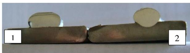
Figure 2 Bead on plate comparisons between (1) GMAW-EM and (2) conventional GMAW processes
