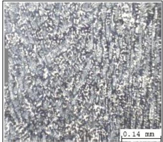
Figure 5 (A) Photomicrograph showing the ferrite morphology in stainless steel weld metal with conventional GMAW process
