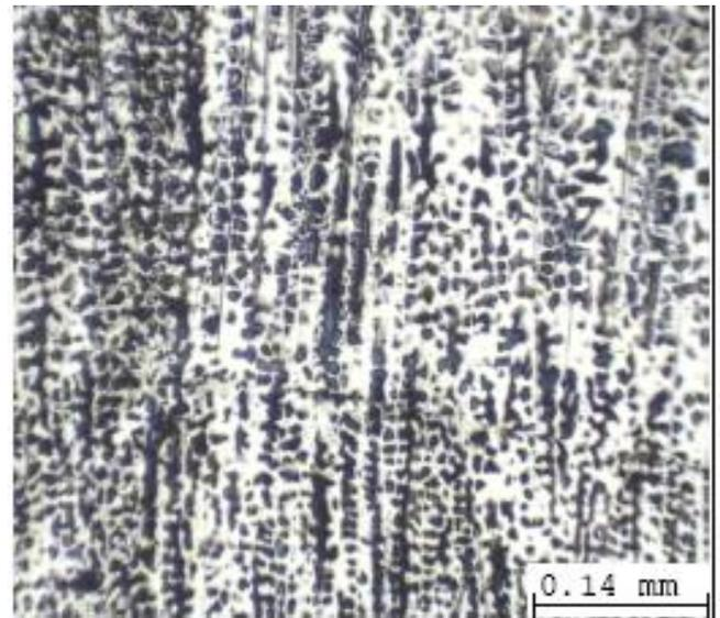
Figure 5 (B) Photomicrograph showing more distinct ferrite morphology in stainless steel weld metal in austenitic matrix of stainless steel weld metal produced with GMAW-EM set up
