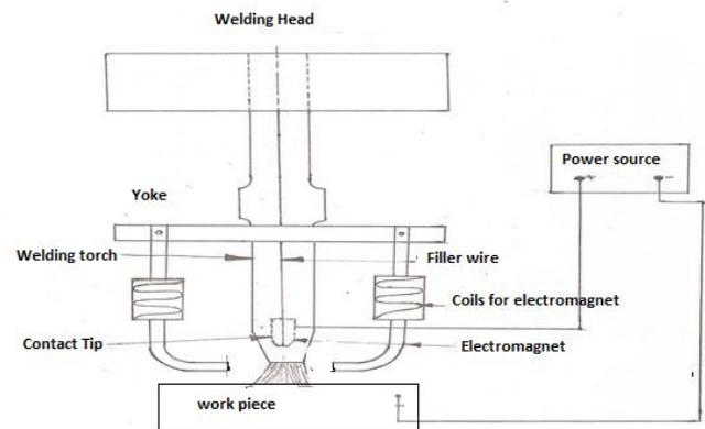
Figure 1 Schematic sketch of GMAW-EM set up
