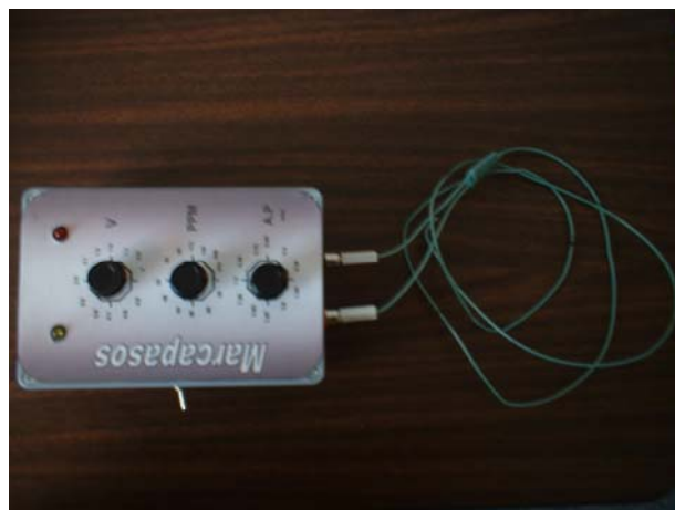
Fig. 6. The pacemaker circuit and electro cater.
