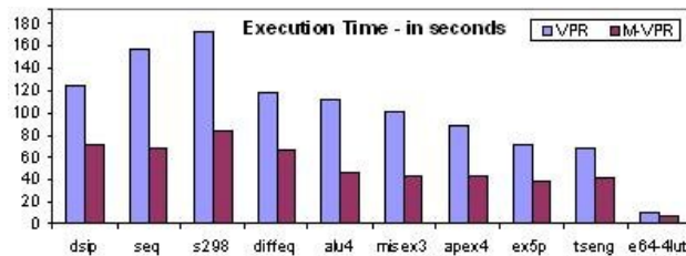
Figure 7: benchmark results in timing-driven placement
