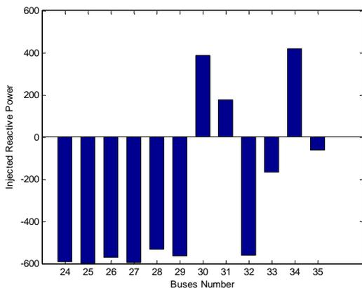
Fig. 6: Bar diagram of injected reactive power to feeders
