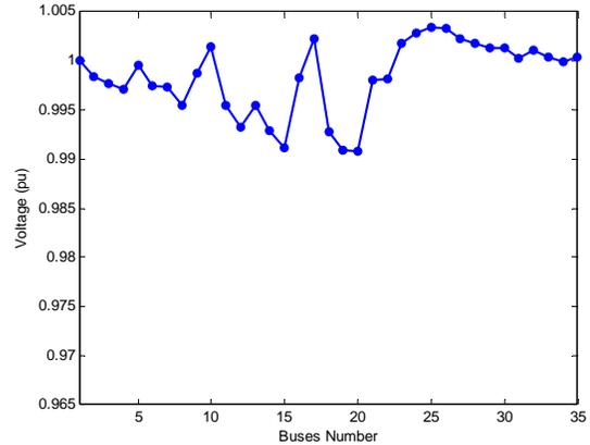
Fig .7: Network voltage profile after reactive power injection
