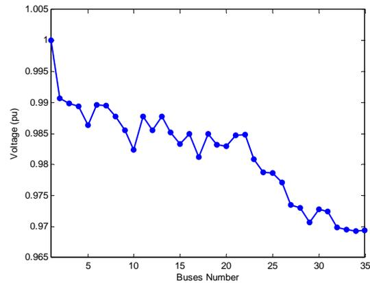
Fig. 3: Initial network voltage profile
