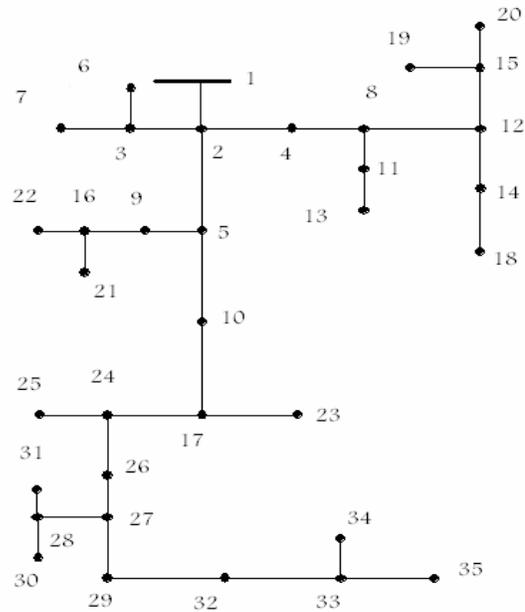
Fig. 2: IEEE modified 35 node test feeder
