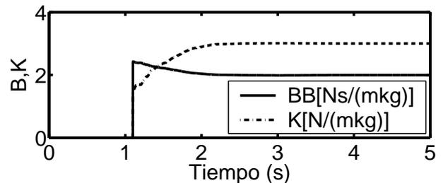
Figure 9: Estimation of B and K with sinusoidal input and noise in the measure of the mass position.
