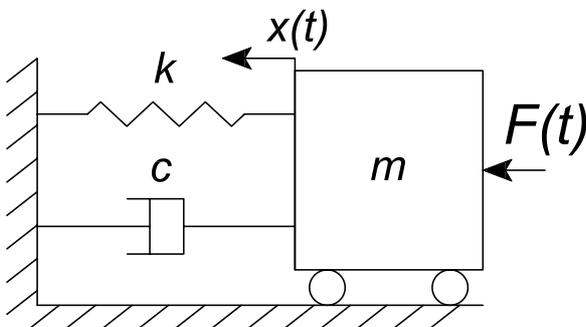
Figure 1: Mass-spring-damper system scheme.
