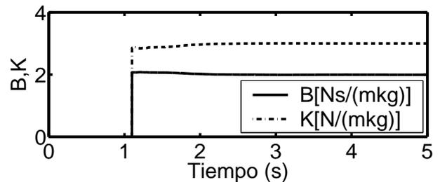
Figure 8: Estimation of B and K with step input and noise in the measure of the mass position.
