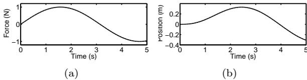
Figure 5: (a) Sinusoidal input to the system. (b) Response of the system to sinusoidal input.
