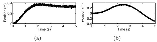
Figure 7: (a) Response of the system to step input and noise in the measure of the mass position. (b) Response of the system to sinusoidal input and error in the measure of the mass position.
