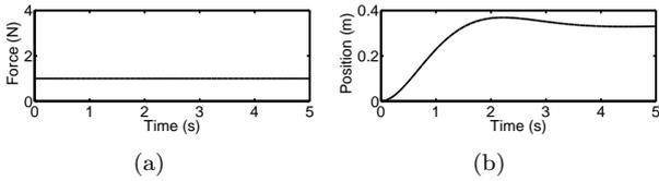
Figure 3: (a) Step input to the system. (b) Response of the system to step input.
