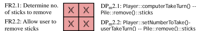
Fig. 6. The two off-diagonal 'X's imply that DP m 2.1 and DP m 2.2 cause an inter-dependency between FR2.1 and FR2.2
