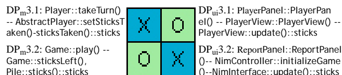
Fig. 8. Absence of off-diagonal 'X's imply that DP_{ui3.1} and DP_{ui3.2} do not cause any dependency between FR3.1 and FR3.2
