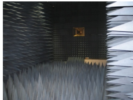
Fig 4. No reflection room where the experiments are performed.
