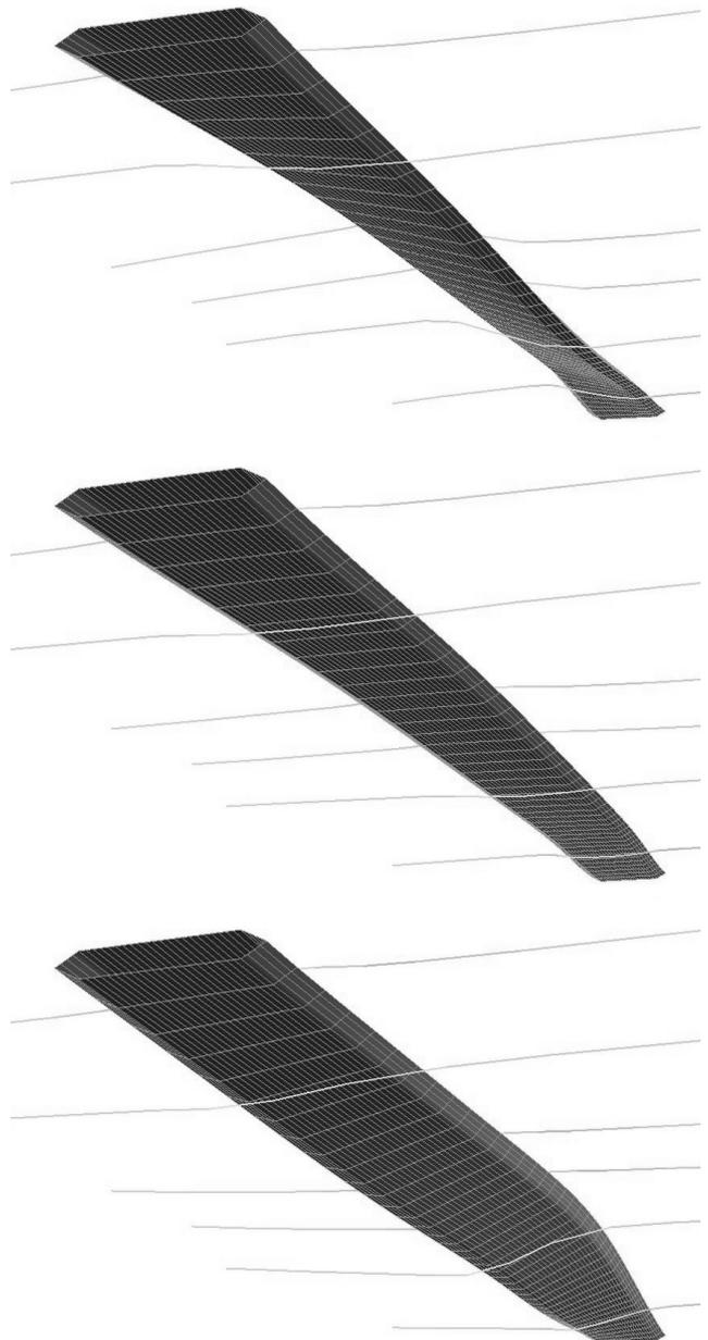
Fig. 8: streamlines around the deformed bridge deck.
