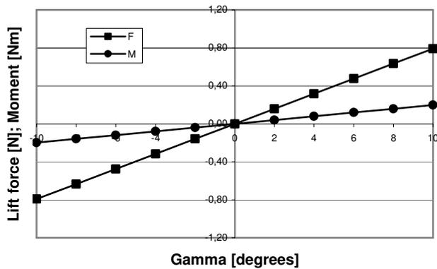
Fig. 9: aerodynamic forces with the flat plate theory.
