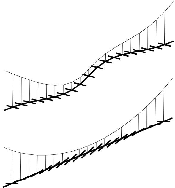
Fig. 11: two mode shapes of the bridge model.
