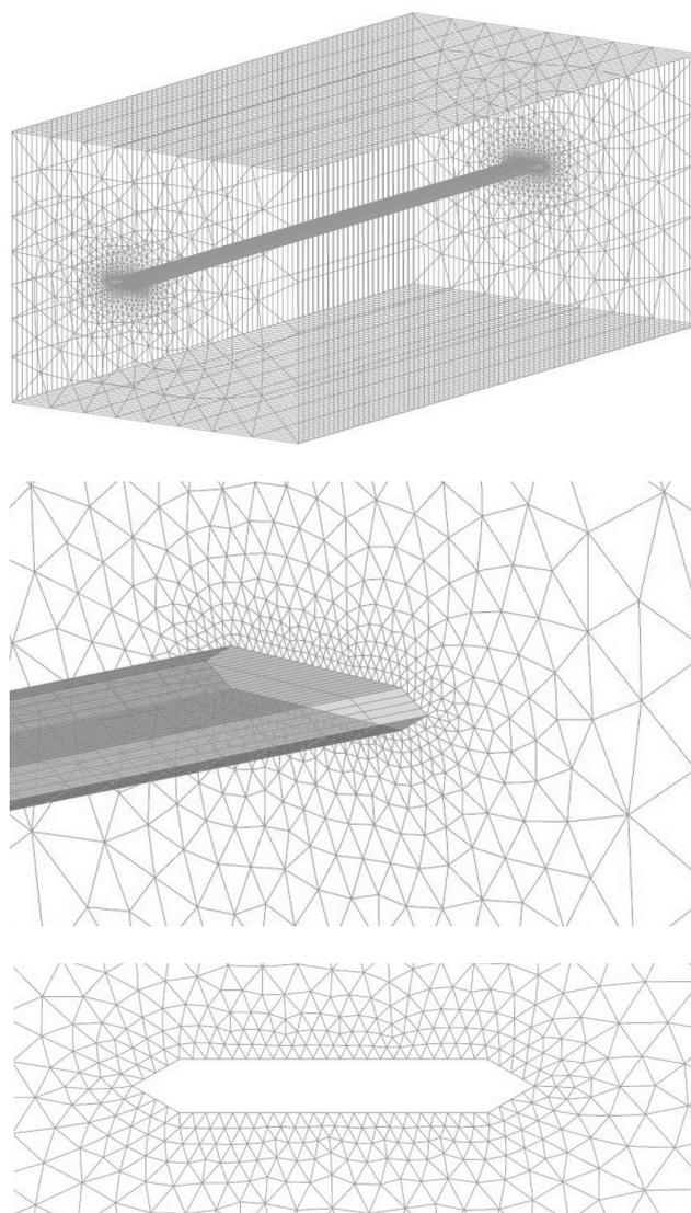
Fig. 6: CFD mesh for the flow simulation.
