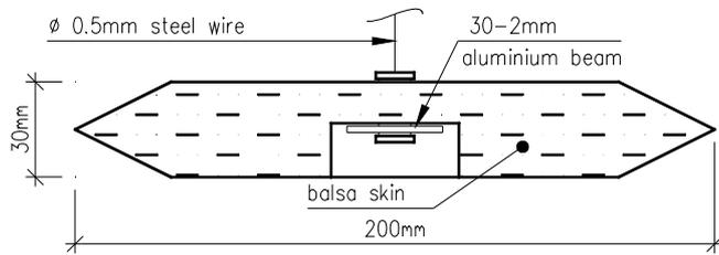
Fig. 3: main dimensions of the wind tunnel model.
