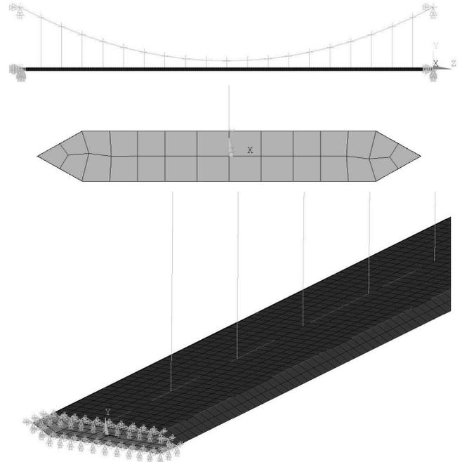
Fig. 4: FEM model details of the bridge.
