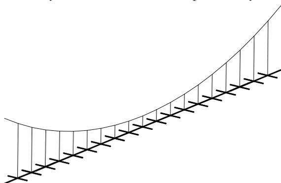
Fig. 10: simplified beam model of the bridge.
