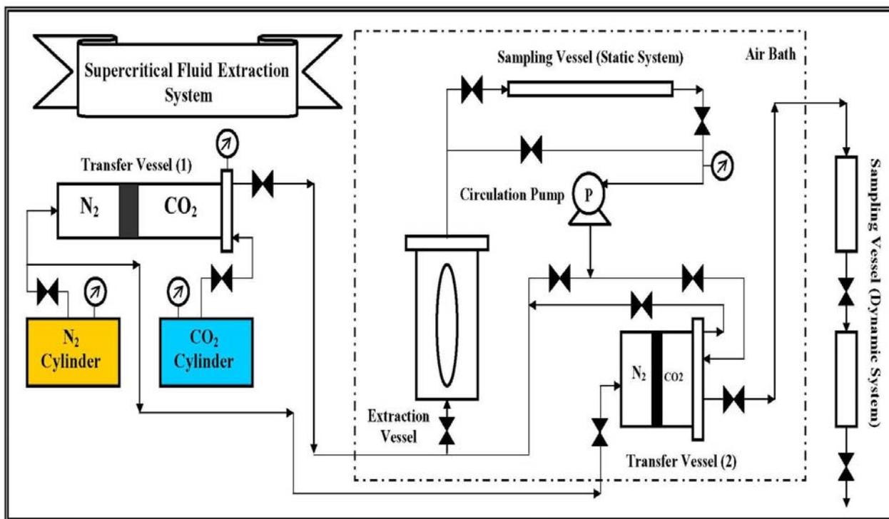
Fig (1). Schematic diagram of the Supercritical Fluid Extraction System (SCFE) for Extraction of oil from canola seed with supercritical carbon dioxide
