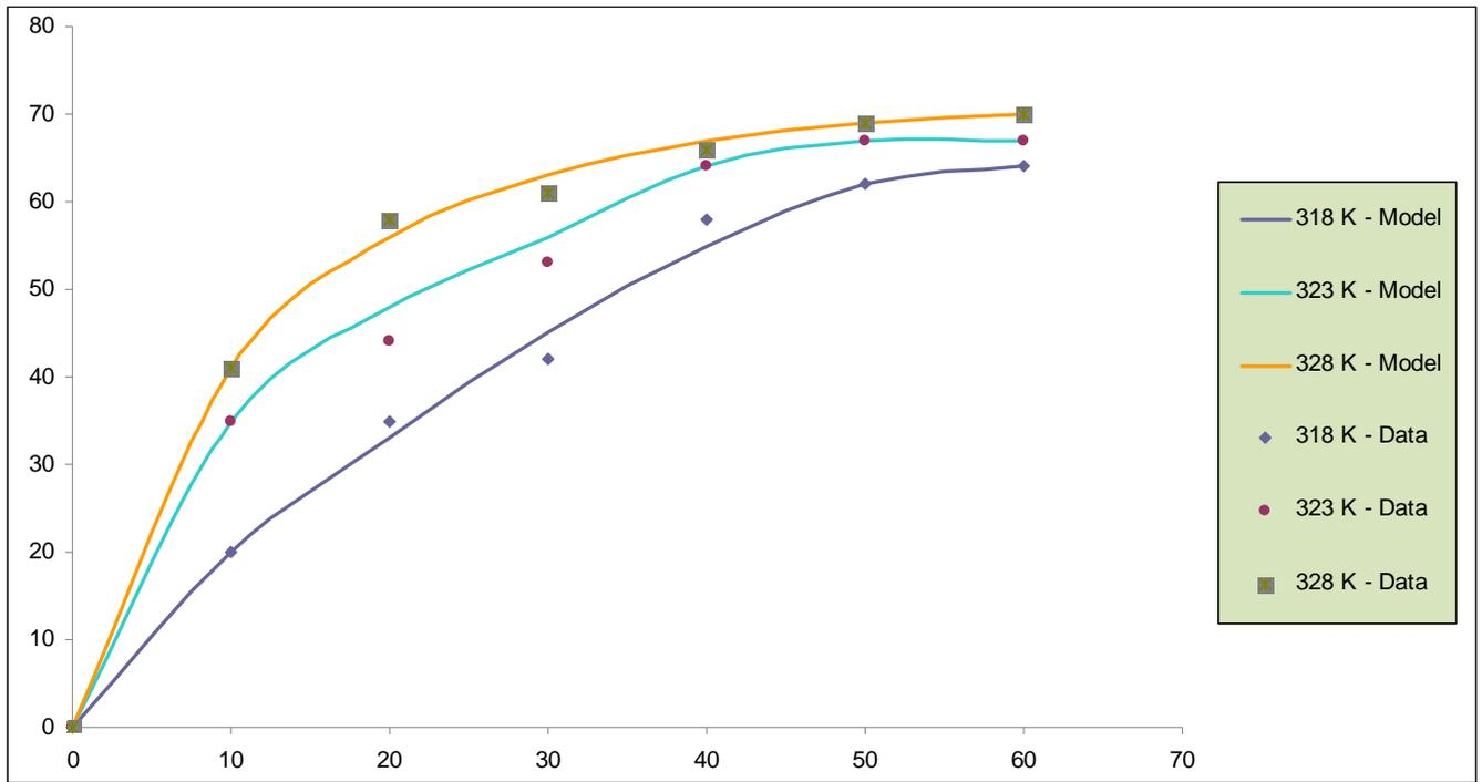
Fig (3): Effect of temperature on the extraction yield of oil at P= 2250 Psi and dp= 0.12 mm
