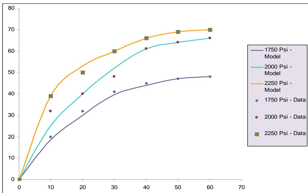
Fig (2): Effect of pressure on the extraction yield of oil at  $T= 328 \text{ K}$  and  $dp = 0.12 \text{ mm}$
