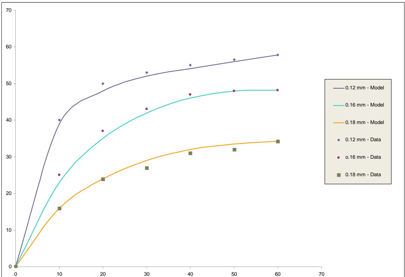
Fig (4): Effect of particle size on the extraction yield of oil at P= 2250 Psi and T= 328 K
