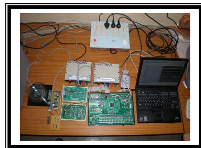
Fig. 6. Photograph of the experimental setup and working model of FPGA based DC motor speed control system
