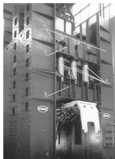
Fig. 3. Stand for testing of powered roof supports located at the KOMAG Institute of Mining Technology.
