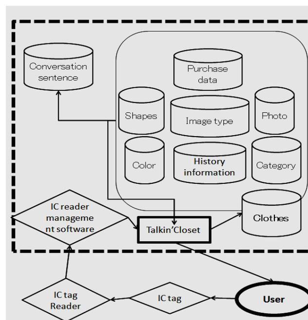
Fig.3. System configuration chart
