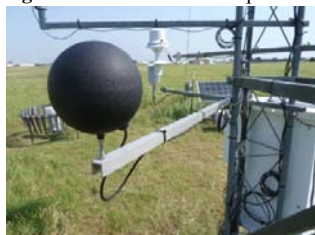
Figure 4. Black Globe Temperature Sensor for Heat Stress used to verify equations at the Oklahoma Mesonet test facility in Norman Oklahoma.
