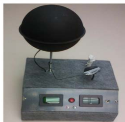
Figure 3. Black Globe Temperature Sensor used in preliminary tests.
