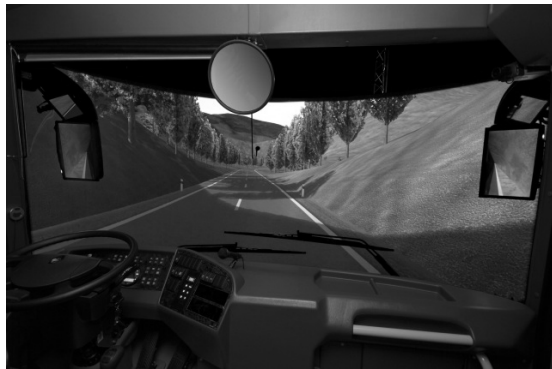
Fig. 2. Simulator with a cylindrical screen - a view of the cabin and the screen with displayed image, from outside and from inside of the cabin.
