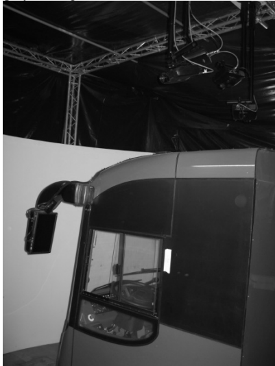
Fig. 3. Simulator with a cylindrical screen - visible cabin, cylindrical screen and projection system.
