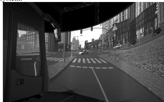
Fig. 1. Simulator with a cylindrical screen - a view of the cabin and the screen with displayed image, from outside and from inside of the cabin.
