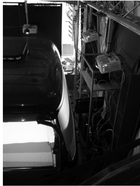
Fig. 4. The test simulator with "on screen" projection - visible cabin with "on screen" screens and projectors that support front and left side windows
