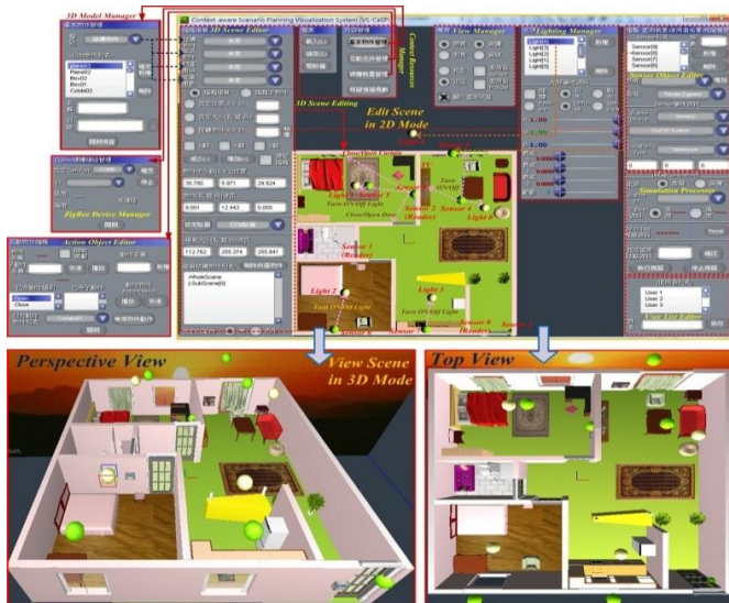
Fig. 6. VS-CaSP system and smart buildings created by 2D/3D methods
