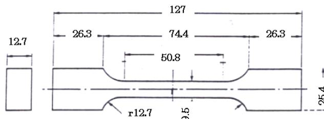
Fig.1 Uniaxial tensile JANNAF testing specimen. (all dimensions: mm)
