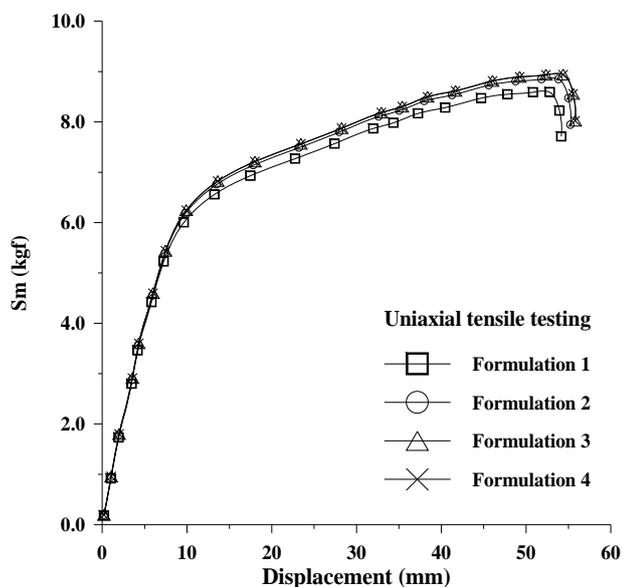
Fig. 4 Uniaxial tensile testing of loading-displacement curve
