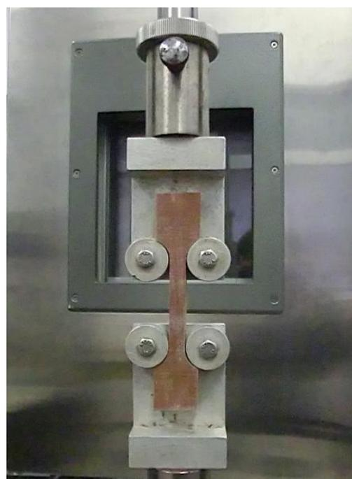
Fig.2 JANNAF specimen with load cell grip.
