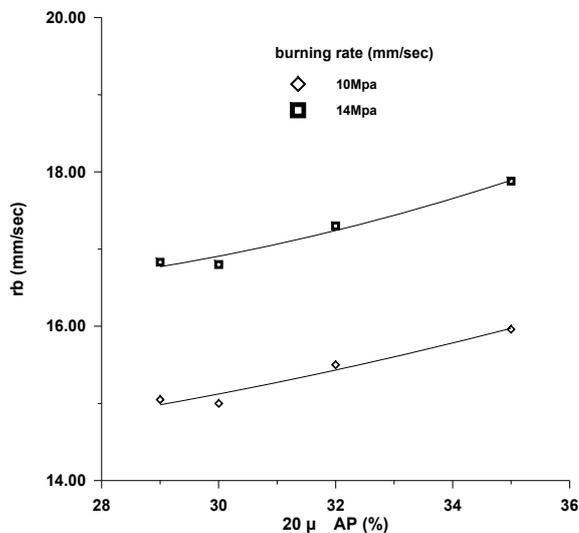
Fig. 5 Variation in propellant burning rate with diverse proportion AP
