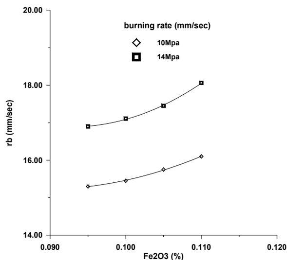
Fig. 5 Variation in propellant burning rate with diverse proportion  $Fe_2O_3$
