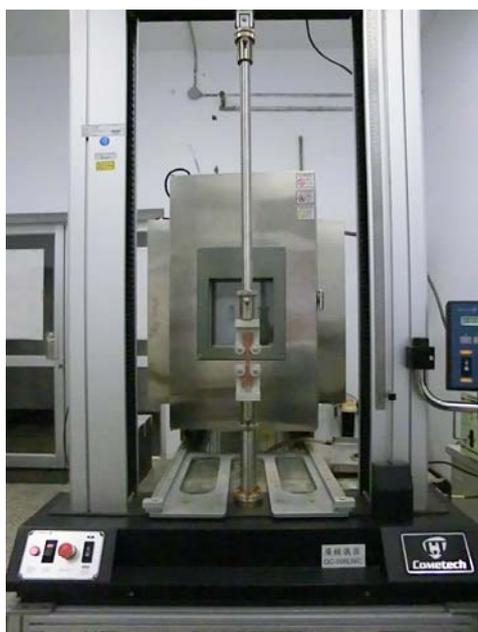
Fig. 3 JANNAF specimen with Cometech QC-506LWC extensometer
