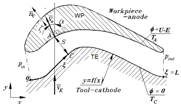
Fig. 5. Schematic the system coordinates and boundary conditions
