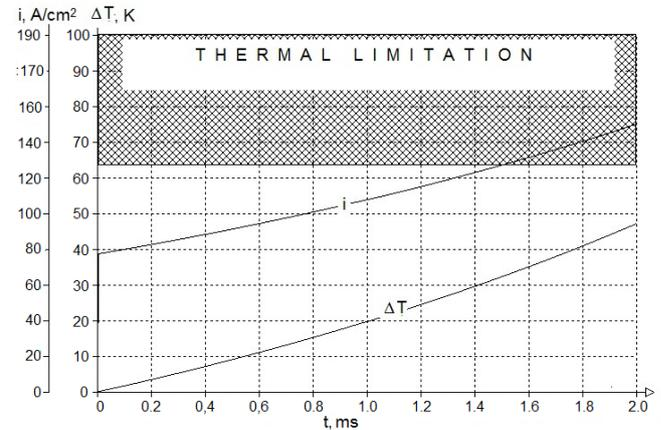
Fig. 8. The current density and the electrolyte temperature changes during pulse on - time in last pulse ( $n=115, m=150$ )
