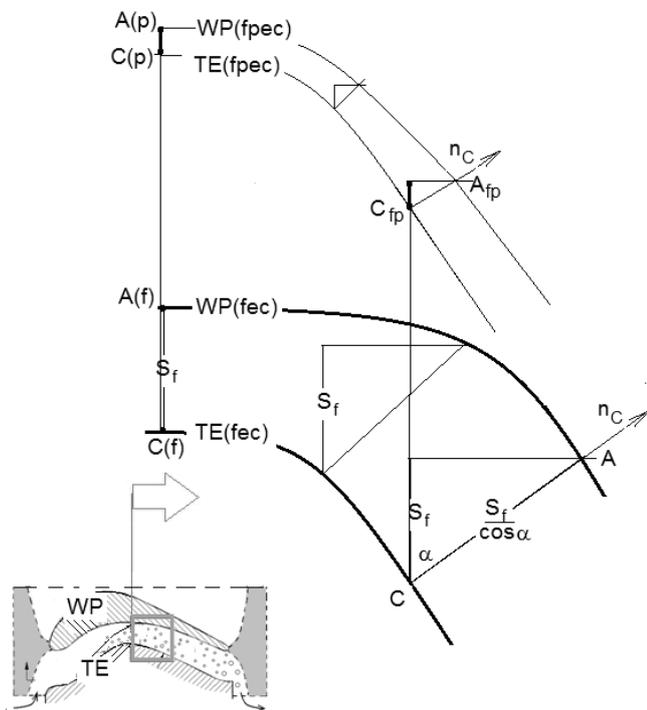
Fig. 7. Scheme of the position of the electrodes: TE(fec) and WP(fec): - the positions of the tool electrode and machined profile respectively, in the final moment of ECM stage and the initial moment of PECM; TE(fpec), WP(fpec) - the positions of TE and WP in the final moment of PECM.
