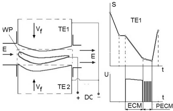
Fig. 6. Principal scheme of the shaping of both side of airfoil with using the sequence of ECM and PECM treatments : TE(1,2)-tool electrodes, WP- workpiece, E - electrolyte, DC - power supply of continuous and pulse current.
