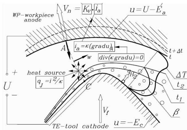
Fig. 4: Schematic diagram of the physical state in the gap :  $i$  - current density,  $U$  - pulse voltage,  $u$  - electrical potential,  $E_a, E_c$  - overpotential on anode and cathode.
