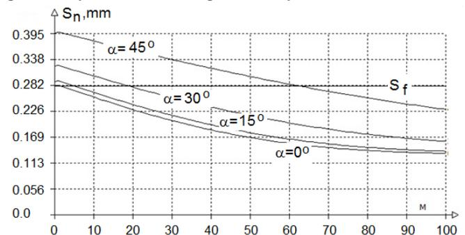
Fig. 9. Changes in the local gap size at different angle during serial pulse pocket M
