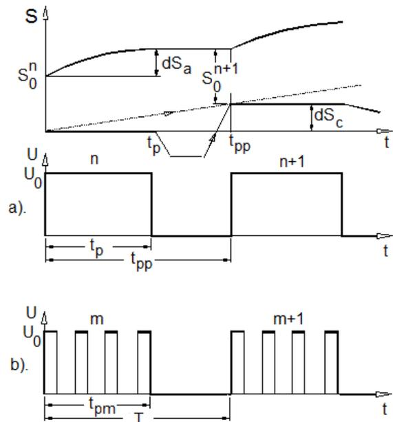
Fig.3. A scheme of PECM with (a) single voltage pulses and (b) pockets/grouped pulses.
