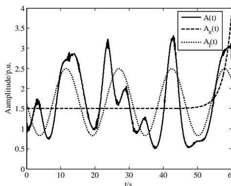
Fig. 6 Instantaneous amplitude of processed active power of G4 in Fa Er
