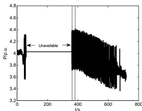
Fig. 5 Active power oscillation of G4 in Fa Er
