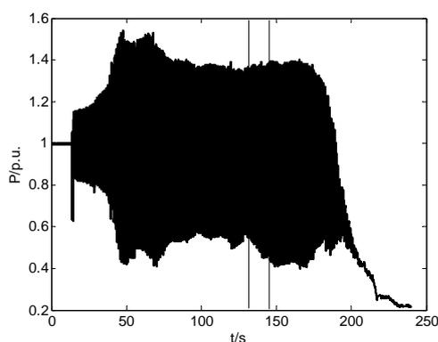
Fig. 3 Active power oscillation of G1 in Ping Ban
