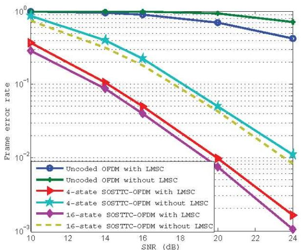
Fig. 8. FER performance of QPSK SOSTTC-OFDM with and without LMSC
