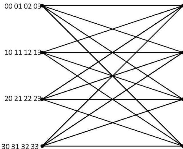
Fig. 2. 4-State QPSK STTC-OFDM Trellis
