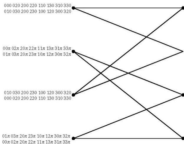
Fig. 4. 4-State QPSK SOSTTC-OFDM Trellis
