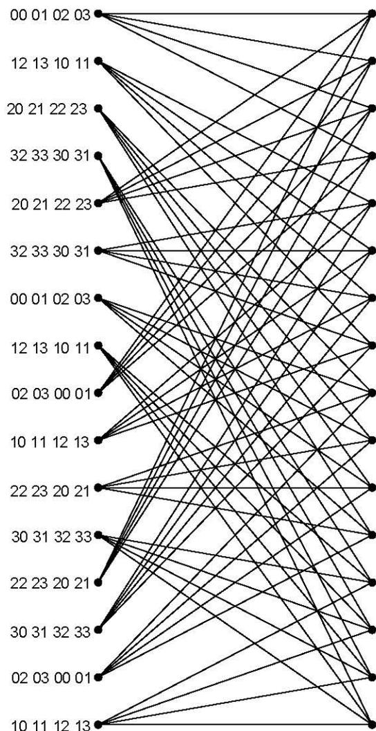
Fig. 3. 16-State QPSK STTC-OFDM Trellis
