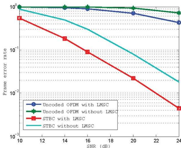
Fig. 6. FER performance of QPSK STBC-OFDM with and without LMSC
