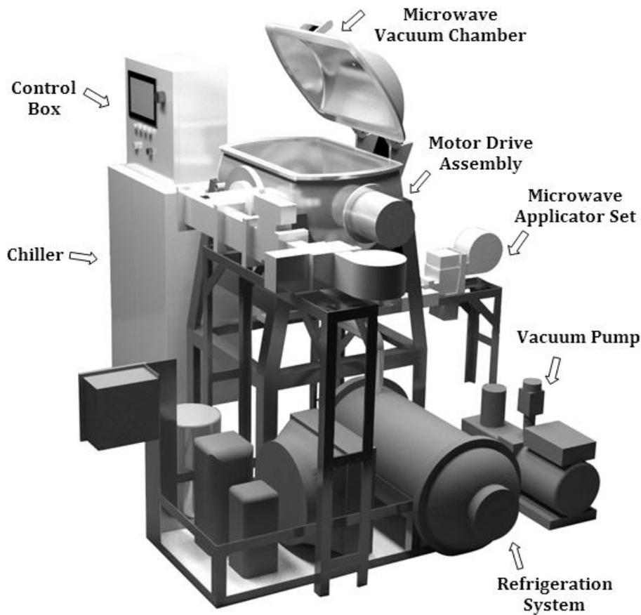
Fig. 6. Complete overview of a microwave vacuum dryer
