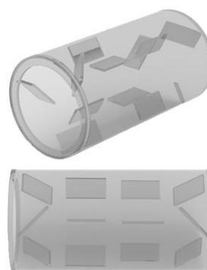
Fig. 3. Design of sample holders with plights
