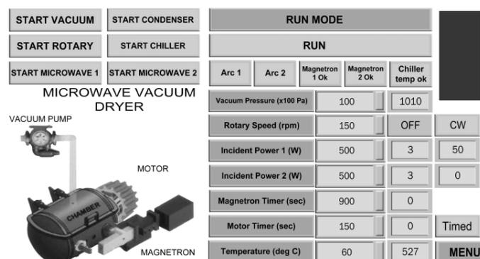
Fig. 5. Setting of drying parameters in the HMI of the control panel box
