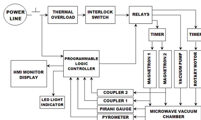
Fig. 4. System block diagram of an MVD
