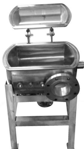
Fig. 1. Fabricated microwave vacuum chamber as the result of the simulations
