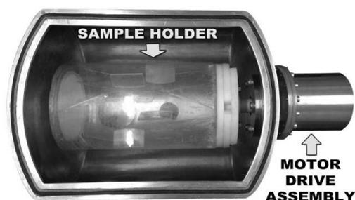
Fig. 2. Attachment of rotary drive assembly to the microwave vacuum chamber
