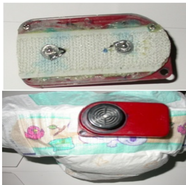
Fig 9. Pressing studs fixed on detector unit & the wet detector unit fixed on the upper front portion of the diaper
