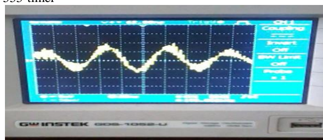
Figure 4: Simulation results of a triangular wave signal by a 555-timer
